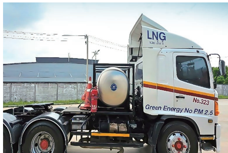
Truck equipped with an LNG tank instead of a CNG tank
